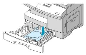
**3** Adjust the rear paper guide to the desired paper length. It is preset to Letter or A4 size depending on the country. To load another size, lift and insert the rear guide into the corresponding position.
